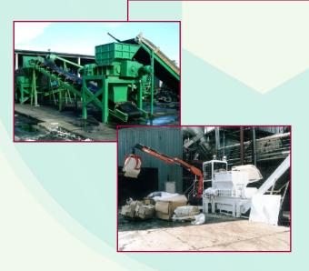
We produce the shredders on the CNC-machines. The output inspection secures the quality of individual components. The stand and feeding hopper are construed with regard to the inclusion of the shredder into the whole complex.
